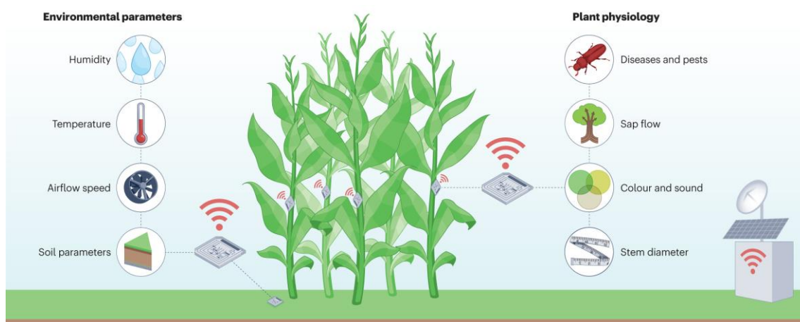
Figure | Envisioned architecture for the Internet of Plants. | Sensor modules comprising environmental sensors, physiological sensors and dedicated electronics for power and communication are distributed throughout the crops and wirelessly connected to a central processor.
